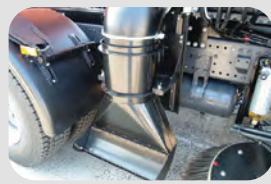
Blower nozzles can be directed manually or from cab
