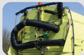
Manual suction system at the rear
